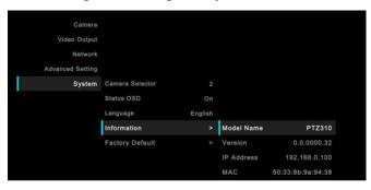
2. Once you have the IP address setup, type the IP address in your Chrome browser (Setup on same subnet) and you should now see the login to the PTZ330 camera shown below.
